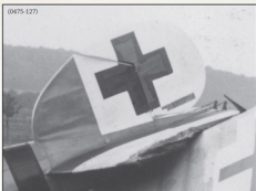
Fin and rudder detail from OAW built Albatros D.Va 6753/17. Note the serial number stenciled onto the lozenge covered rudder which has been carefully painted around when the white was applied to the rudder at the unidentified unit.
