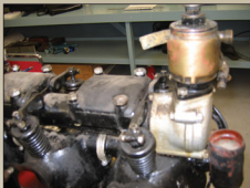
Thick air pump (E29) characteristic of the 180hp Daimler-Mercedes D.IIIa. Note the rocker boxes (E27) are now positioned to the rear of the springs.
