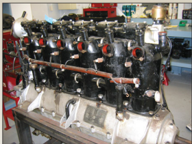
Right side of the engine. Note the water pipe running through the cylinders and the position of the data plate.
